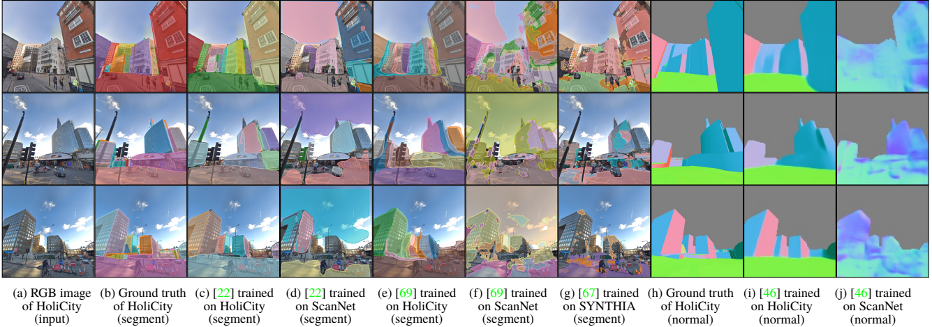
Figure 4: Qualitative results of models evaluated on HoliCity. We test models of MaskRCNN [22], Associative Embedding [69], PlaneRecover [67], and UNet [46] that are trained on HoliCity, ScanNet [14], and SYNTHIA [47] on HoliCity.
