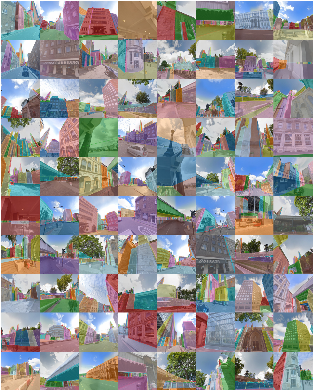
Figure 7: Random sampled perspective images overlaid with surface segments from high-resolution CAD models.
