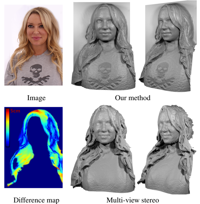
Figure 11: Comparison with multi-view stereo. Our single-view reconstruction result closely matches the result of the state-of-the-art multi-view stereo method [Fuhrmann et al. 2014] on a multi-view dataset (with an average difference of 2cm) and preserves more coherent and detailed hair structures.
