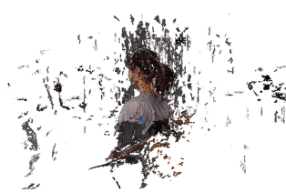
Figure 3: Initial point cloud reconstructed from multi-view stereo with outliers.
