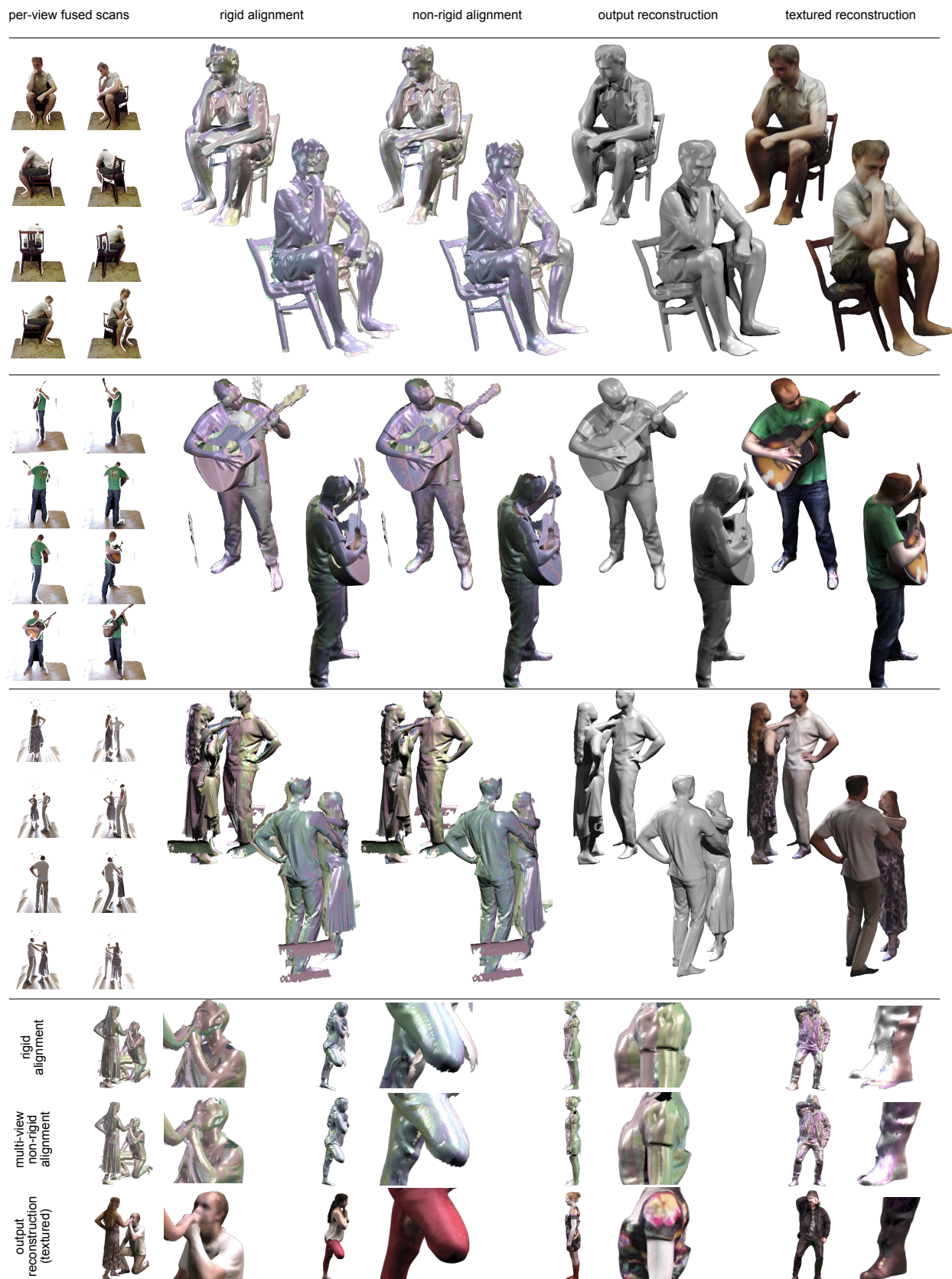
Figure 15: Example 3D self-portraits captured by our system. For each example we show the input raw scans, the initial scans registered by rigid alignment, the scans refined by multi-view non-rigid alignment, the merged surfaces and reconstructed textures. Using only a single static Kinect sensor, our algorithm successfully reconstructs textured geometry of challenging examples (arbitrary poses, subjects with props, loose clothing, multiple subjects, etc.). While being more general and efficient than existing methods, our system can also handle inconsistent illuminations across views and is particularly robust to large deformations.
